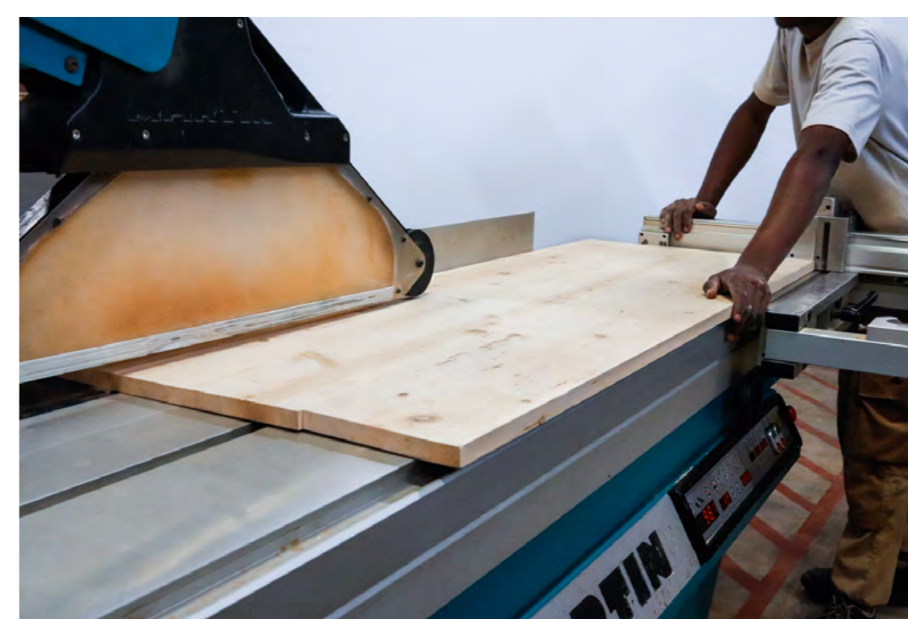
Protection device and hand position for inset cutting. The saw blade will be lifted trough the workpiece.
