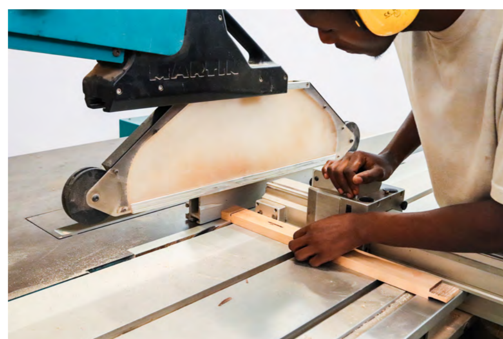
Protection device and hand position for cutting tenons.
