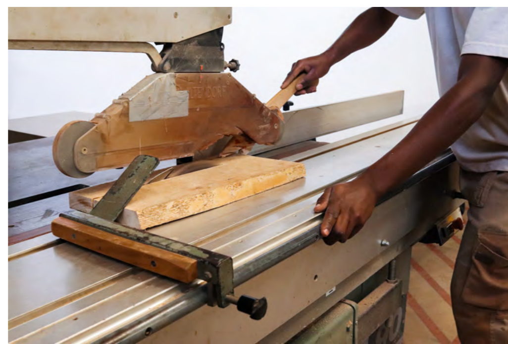
Rip cutting of smaller pieces with the push-stick.
