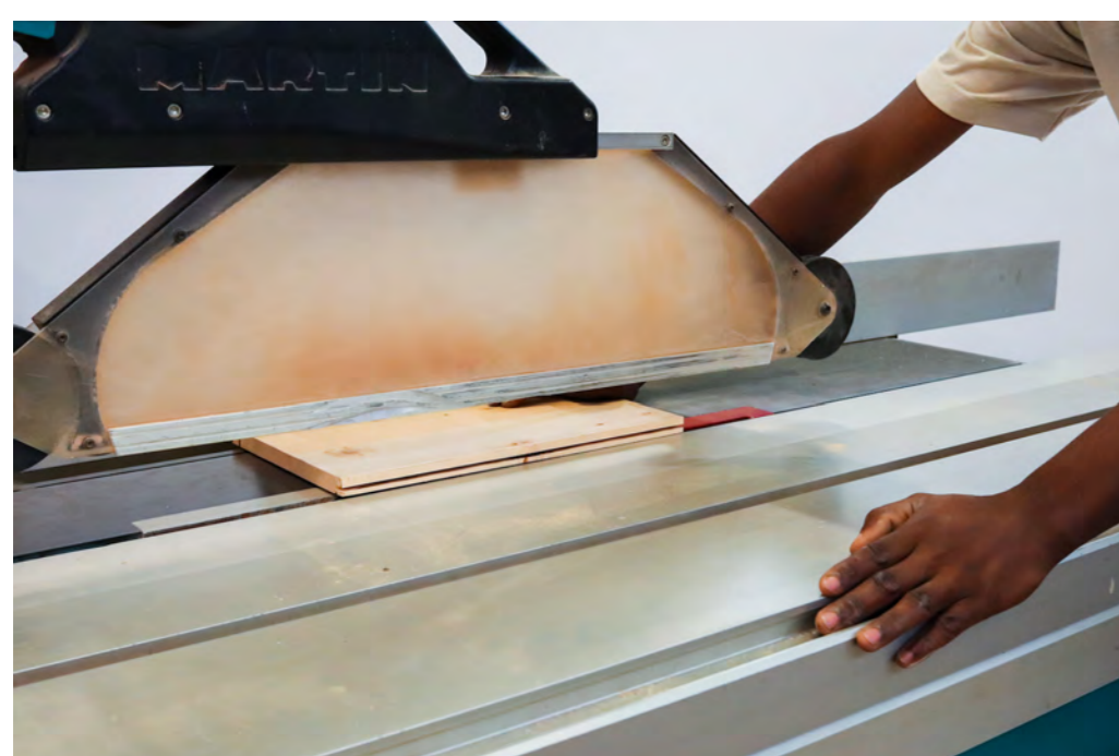
Protection device and hand position for cutting rabbets.
