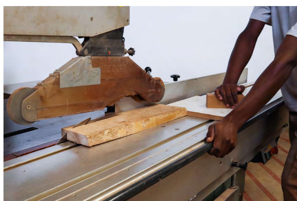
Rip cutting of strips with a push block.
