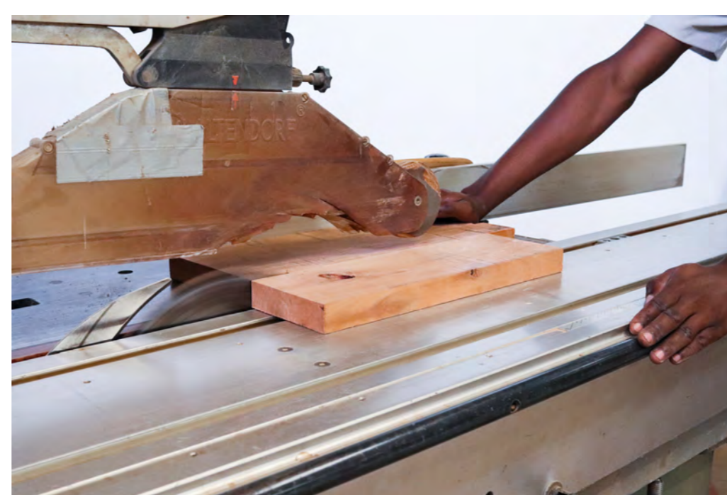
Rip cutting by hand (width over 120mm).
