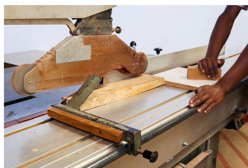
Rip cutting of strips with front and back cutting aids.
