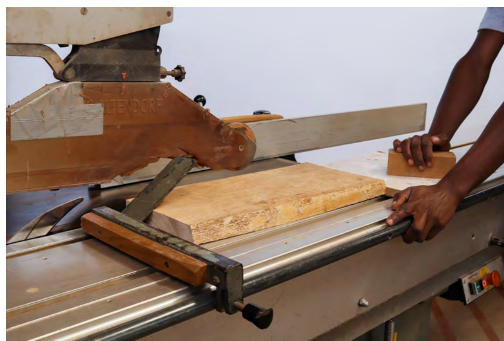
Pull back the rip fence to avoid a clamping of the piece.
