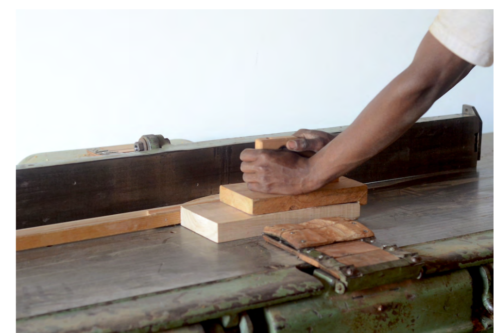
Planing of short workpieces with jointer ledger, folding guard and push block.
