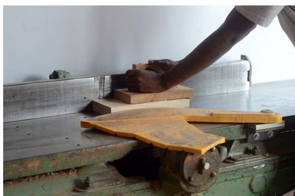
Planing of short workpieces with pivoting protection and push block.
