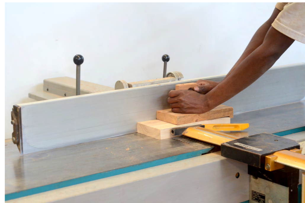
Planing of short workpieces with safety bridge and push block.
