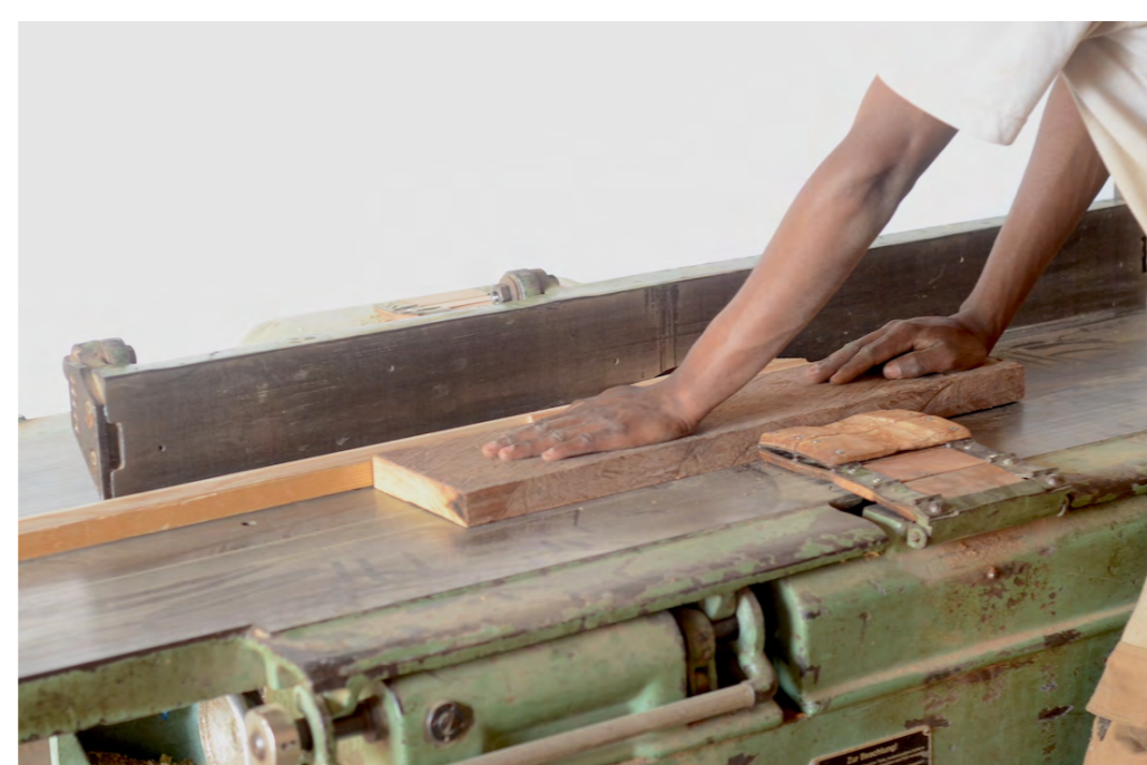
Planing of wide workpieces with jointer ledger and folding guard.
