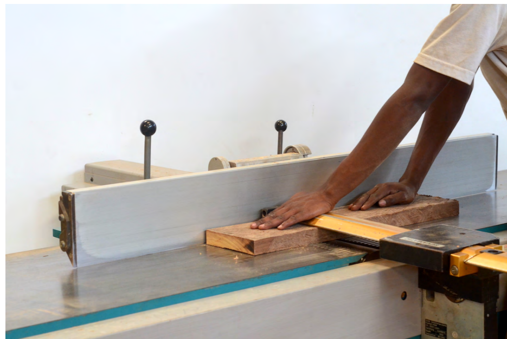
Planing of wide pieces with safety bridge.
