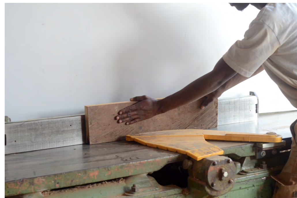
Jointing of wide workpieces with pivoting protection.
