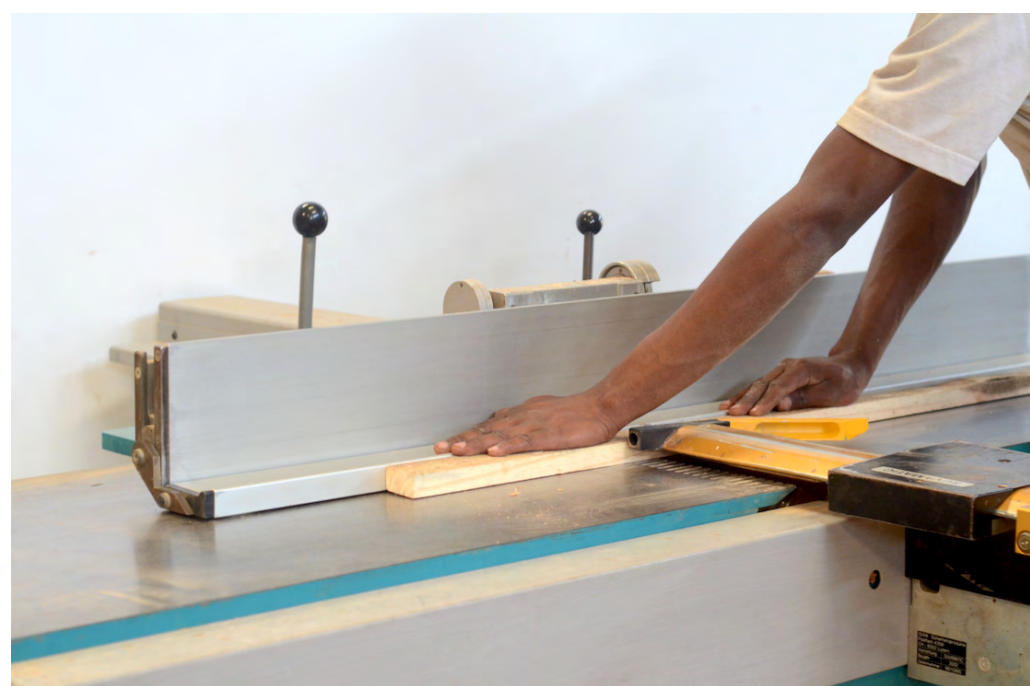
Planing and jointing of narrow pieces with safety bridge and pivoting parallel fence.
