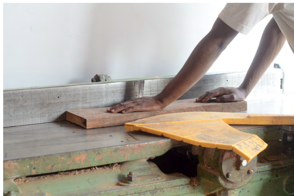
Planing of wide workpieces with pivoting protection.
