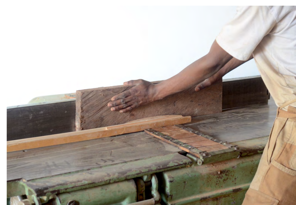
Jointing of wide workpieces with jointer ledger and folding guard.
