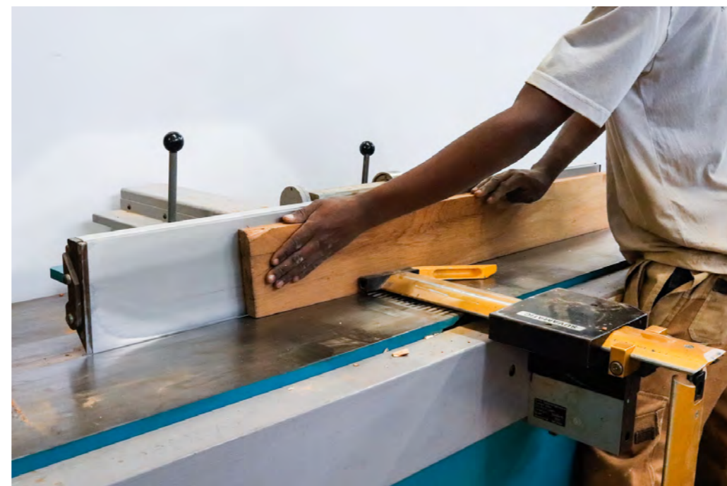
Jointing of wide workpieces with safety bridge.
