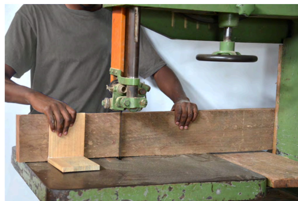
Cross cutting of upended pieces using the machine stand and a square as support
