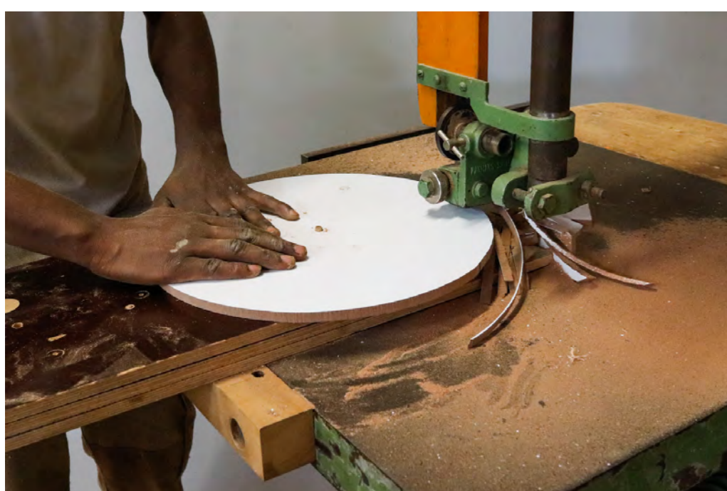
Device and hand position for cutting round panels.
