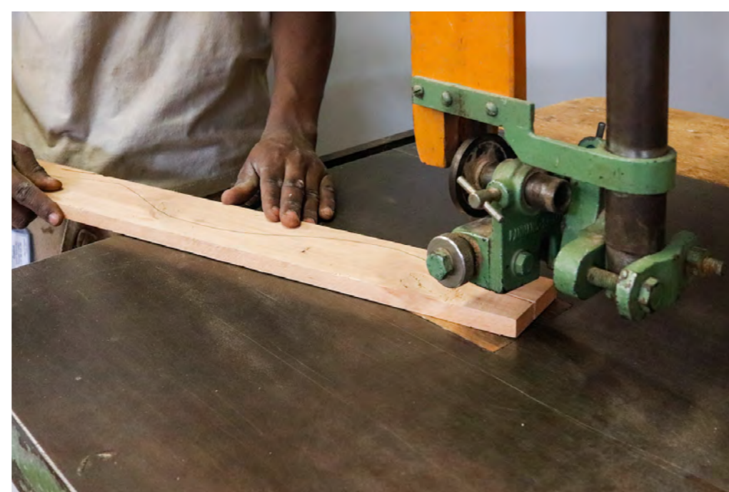
Hand position while cutting curves.
