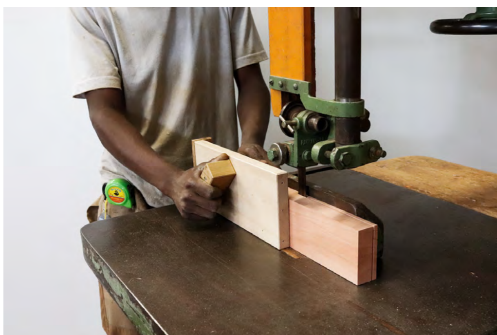
Rip cutting of upright pieces with fence and push block
