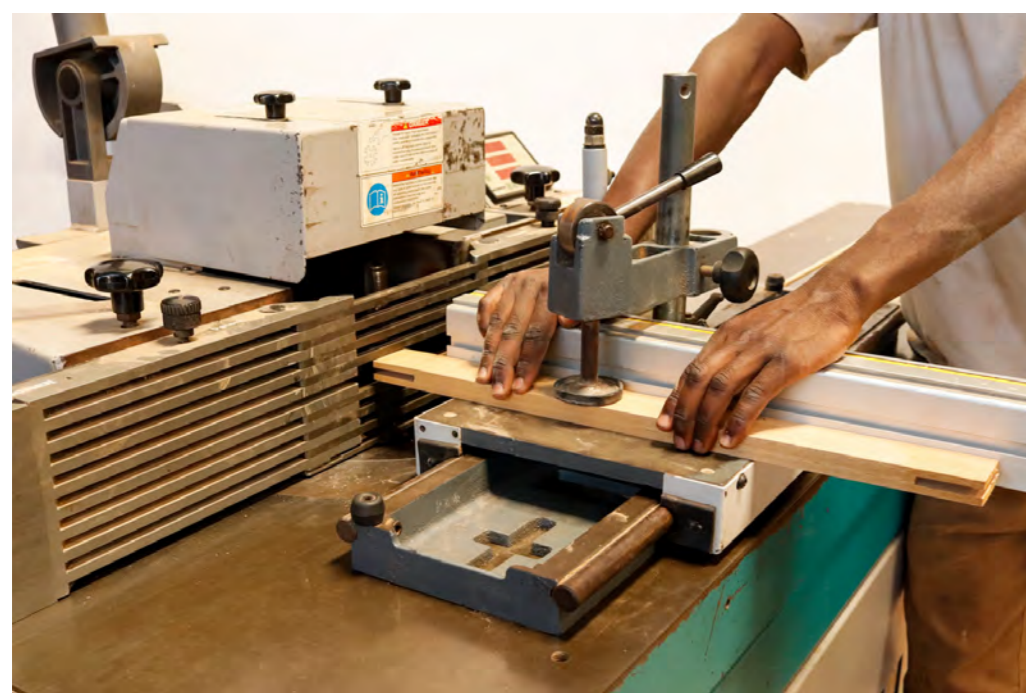
Routing of short edges with sliding fence.
