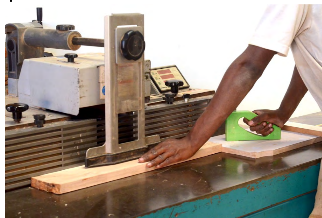
Routing of small pieces at the router fence with cutter guard and push block.
