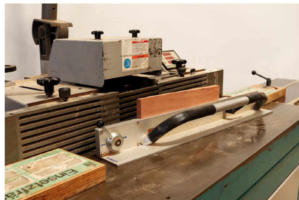
Inset routing of small pieces with clamp strip and kickback protection.
