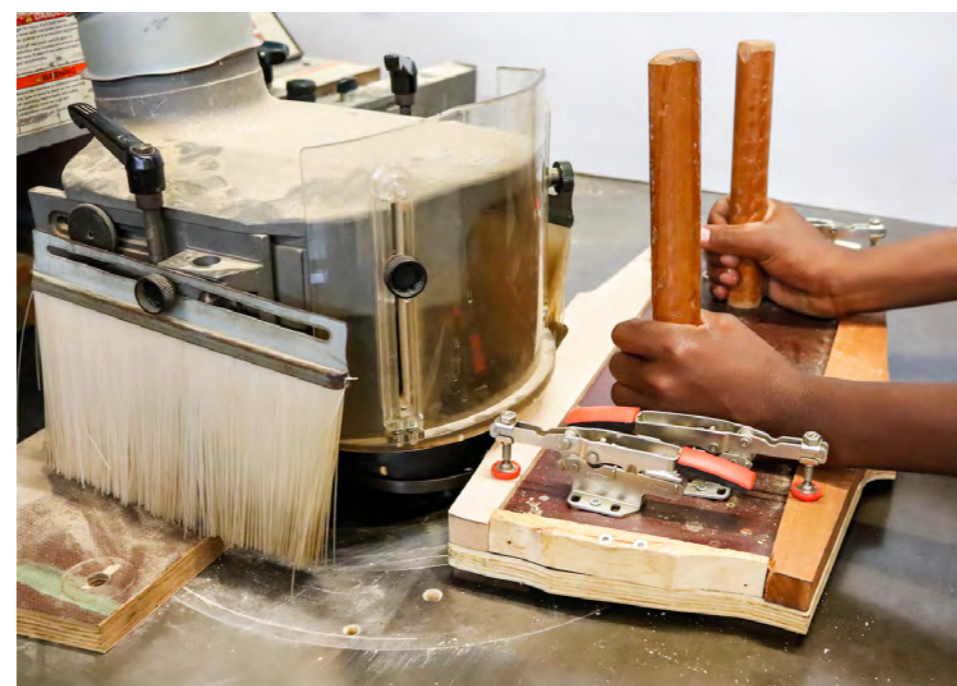
Routing of curved pieces with the copy ring and the round cutter guard – Copy-ring down.
